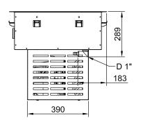
D = Drain El = Electrical inlet (power)
